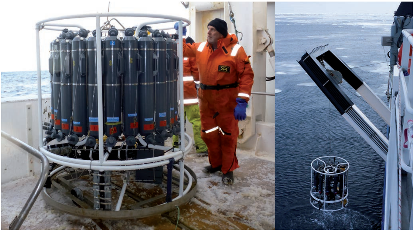
NIWA's Ian Smith guides the CTD (Conductivity, Temperature, Depth) profiler back on board Tangaroa after it has been sampling salinity, pressure, oxygen and temperature to and from the seafloor. The CTD is deployed from the side of the vessel as seen at the right. (Helen Bostock, Eva Cougnon)
