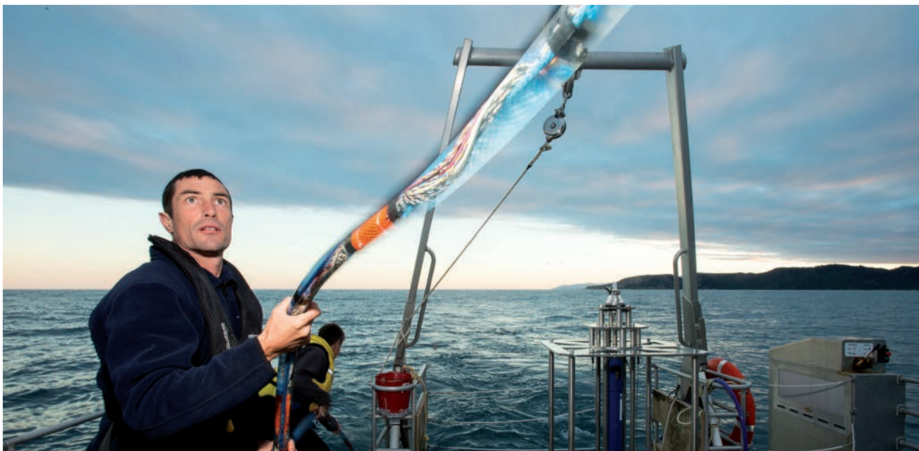
Dr Joshu Mountjoy preparing the applied acoustics boomer and hydrophone for operation off Kaikoura. (Dave Allen)
