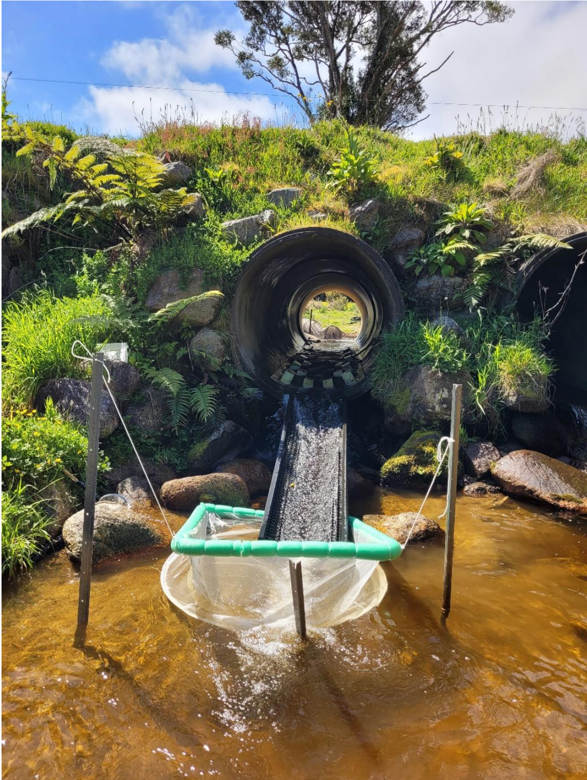
Figure 8-11: Sock net used to create a pool downstream of a floating ramp to hold test fish within. Photo credit: Sjaan Bowie.
