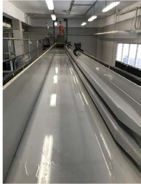
Figure J-6: Examples of longitudinal baffles. Photo credit: Craig Franklin & Rebecca Cramp, University of Queensland.
