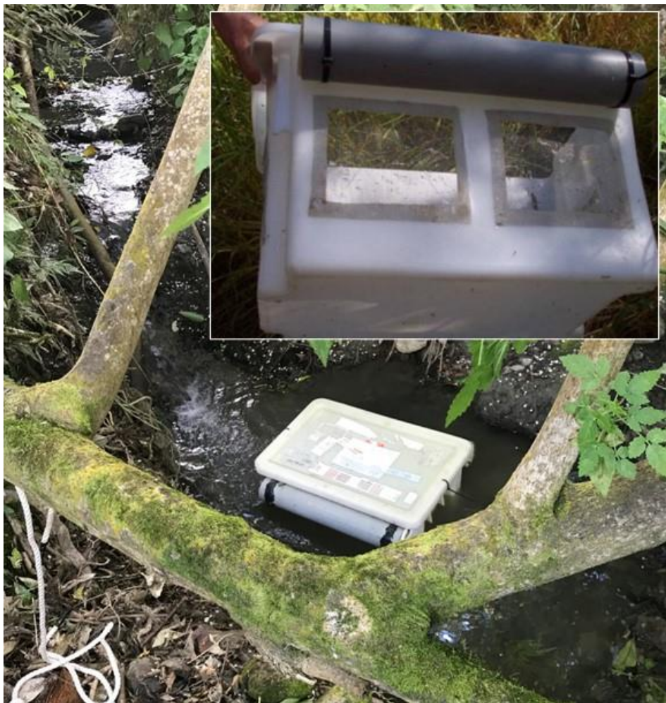
Figure 6-7: Live-bin deployed to maintain īnanga for fish passage trials. Inset shows close up of live-bin.
