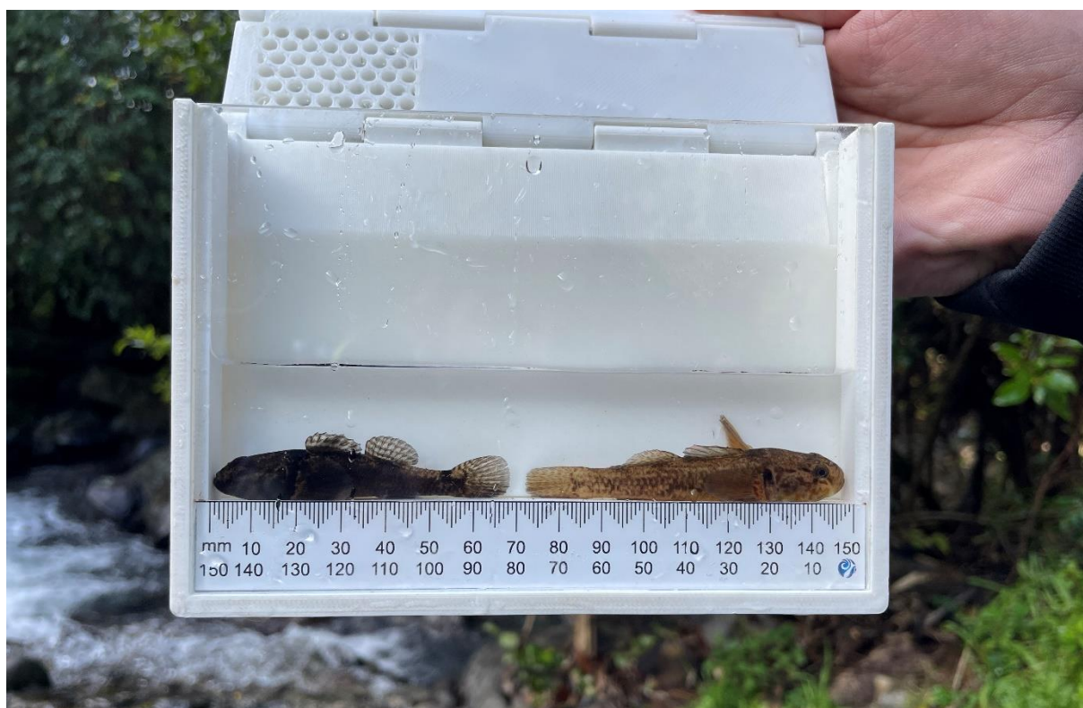
Figure 7-1: NIWA Photarium that can be used to identify fish species and measure their length without anaesthetic.
