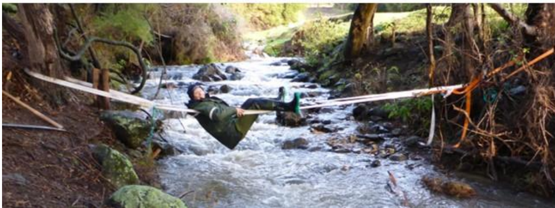
Figure 6-18: Spaced double coil PIT antenna design. Coils have the same orientation with a spacing of 0.4 m. The antenna width (A to B) can be up to 10 m in length. The base of each coil followed the contours of the stream channel with a maximum height of 1.35 m for antenna <10 m in length. For antenna >10 m in length, the maximum height cannot exceed 1 m. The antenna wires should be strongly secured (e.g., with tiedown straps as pictured) but can remain flexible. Abbreviations: AWG, American wire gauge. Figure modified from Baker et al. (2017).
