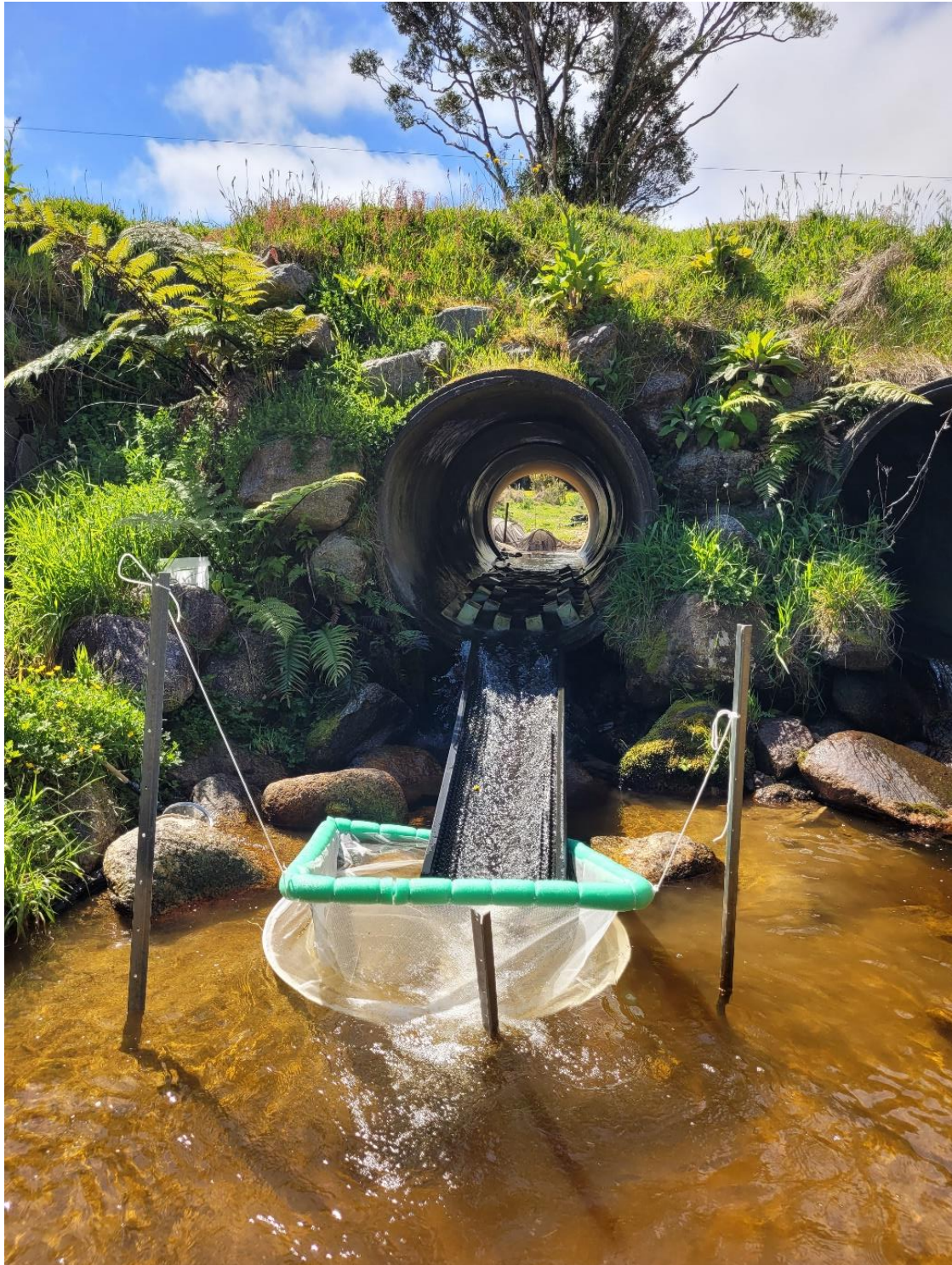
Figure 6-9: Sock net used to create a pool downstream of a floating ramp to hold test fish within. Photo: Sjaan Bowie.
