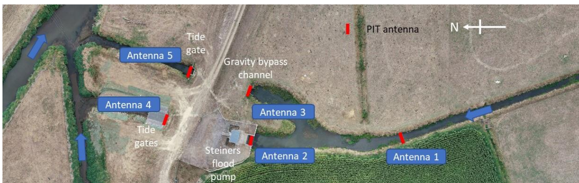
Figure 6-15: Passive Integrated Transponder (PIT) antenna setup at Steiners flood pump station with a gravity bypass. Blue arrows indicate direction of flow. Figure modified from Mahlum et al. (2022).
