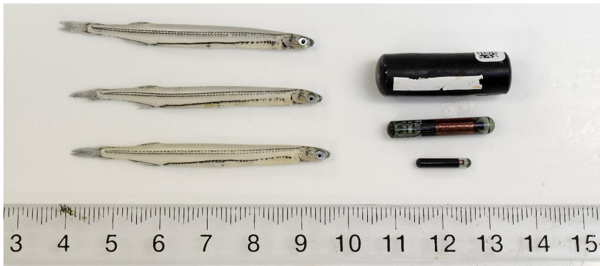
Figure 5-2: Application of biotelemetry methods to the study of many migratory species/life stages in New Zealand is limited by relative tag size. Juvenile galaxiids alongside an acoustic tag (top) and 23 mm (middle) and 12 mm (bottom) HDX PIT tags.
