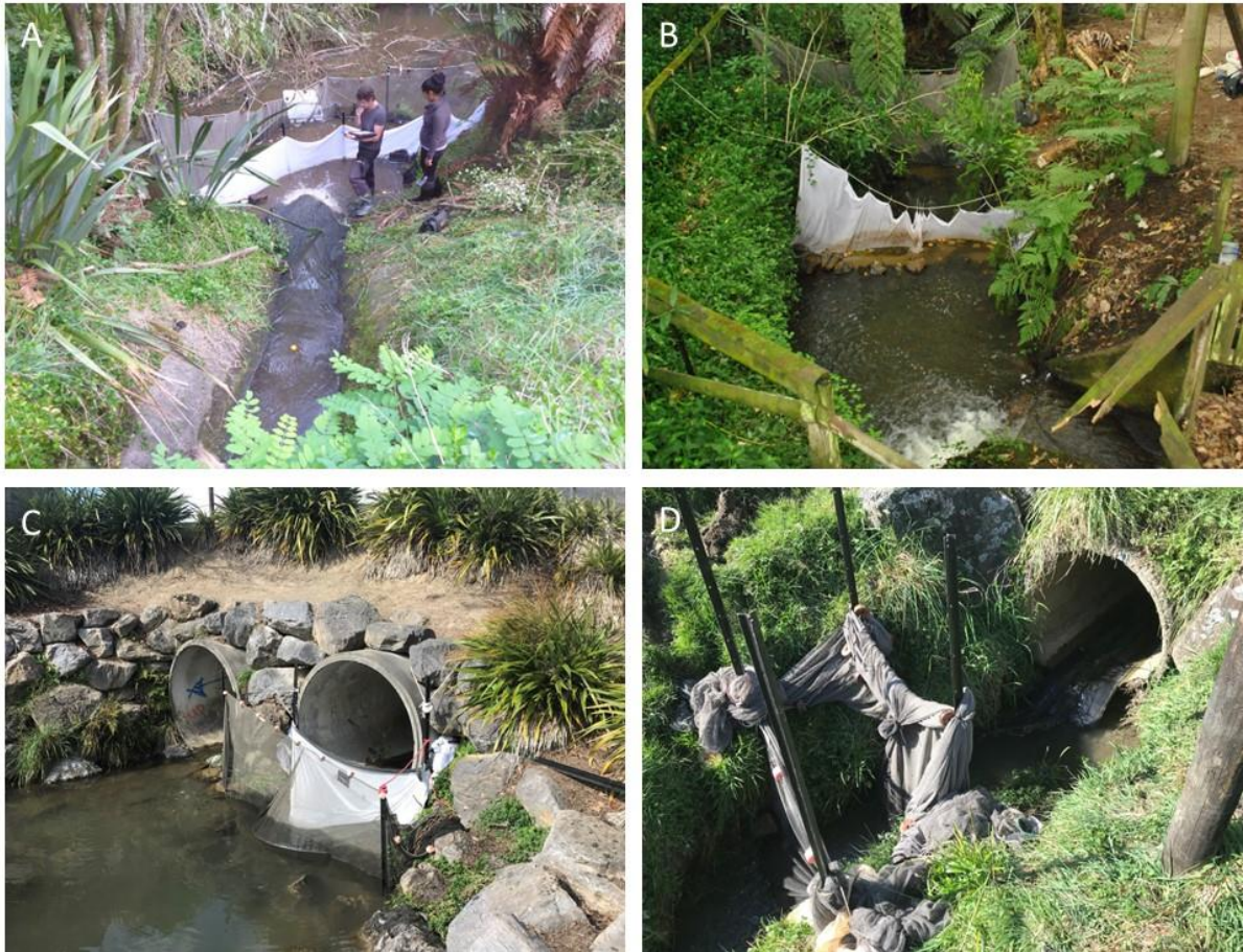
Figure 6-10: Downstream (bottom end of the test site) barricades installed across a range of study sites. A) Mangakotukutuku Stream, Hamilton. B) Bankwood Stram, Wymer Terrace, Hamilton. C) Reservoir Creek, Tasman. D) Oldham Creek, Nelson.
