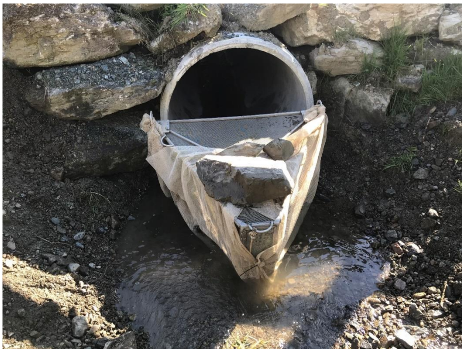
Figure 6-11: Whitebait trap installed at the culvert inlet (top end of the test site) in Oldham Creek.
