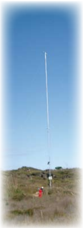
Portable wind-monitoring station in Northland.
