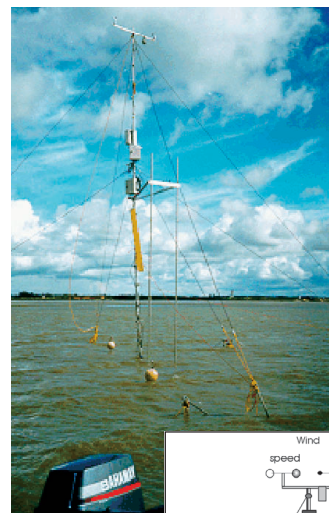
One of the recording sites – on a calm day. The diagram shows some of the instruments used: wave gauges, current meters (S4), current profiler (ADCP), and meteorological sensors.
