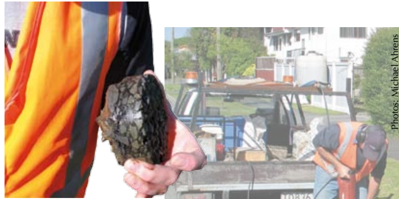
Coring a sample from a Christchurch road. Back in the lab, the different layers of seal are clearly visible in a section of the core.
