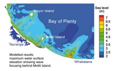
height in the central portion is 5.4 m onshore from Motiti Island, arriving about 70 minutes after fault rupture. Waves breach the coastal sand dunes at this location.
