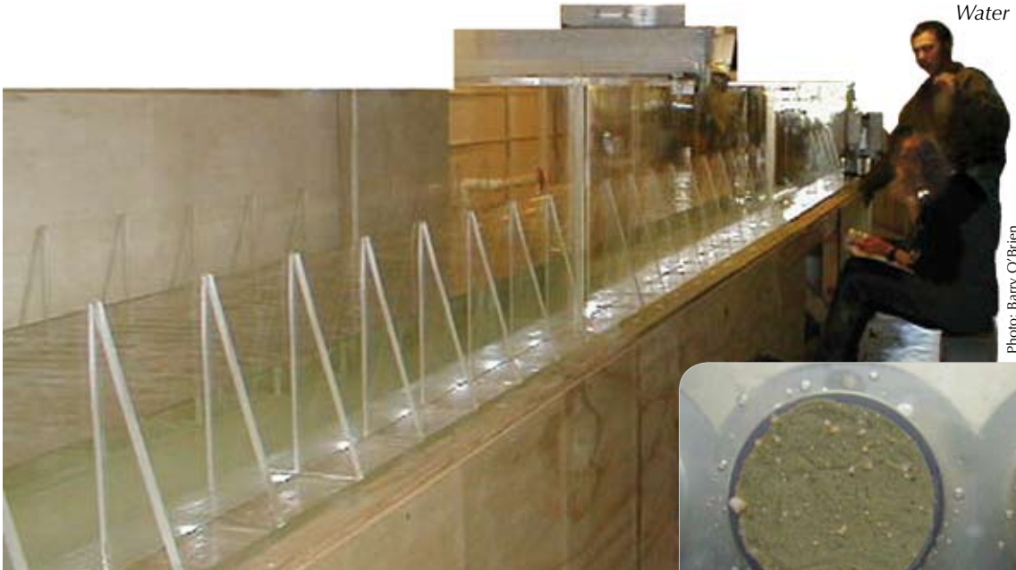
The laboratory flume, located at the University of Waikato, Department of Biological Sciences. The flume is 7.23 m long by 50 cm wide; the working area is 0.9 m long. Water is recirculated through the flume by a propeller located in a return pipe at the end of the channel.
