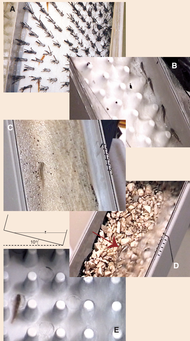
Ramp surfaces tested. A , bristles, showing 3 redfin bullies climbing the wetted margin. B , egg carton, showing 4 redfin bullies climbing the wetted margin. C , sand, with an inanga resting on wetted margin. D , gravel, arrow points to an inanga resting on wetted margin. E , stripdrain, showing a redfin bully climbing the wetted margin. The ramps are tilted (as shown in the inset diagram) so the wetted margin is on the left-hand side of the ramp (A, C, D and E) or on the right (B).
