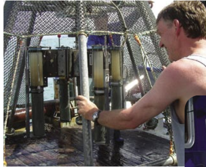
Peter Gerring wrangles the multi-corer onboard RV Kaharoa. Kim Currie sets up sediment incubation experiments for measuring nutrient fluxes and denitrification rates.
