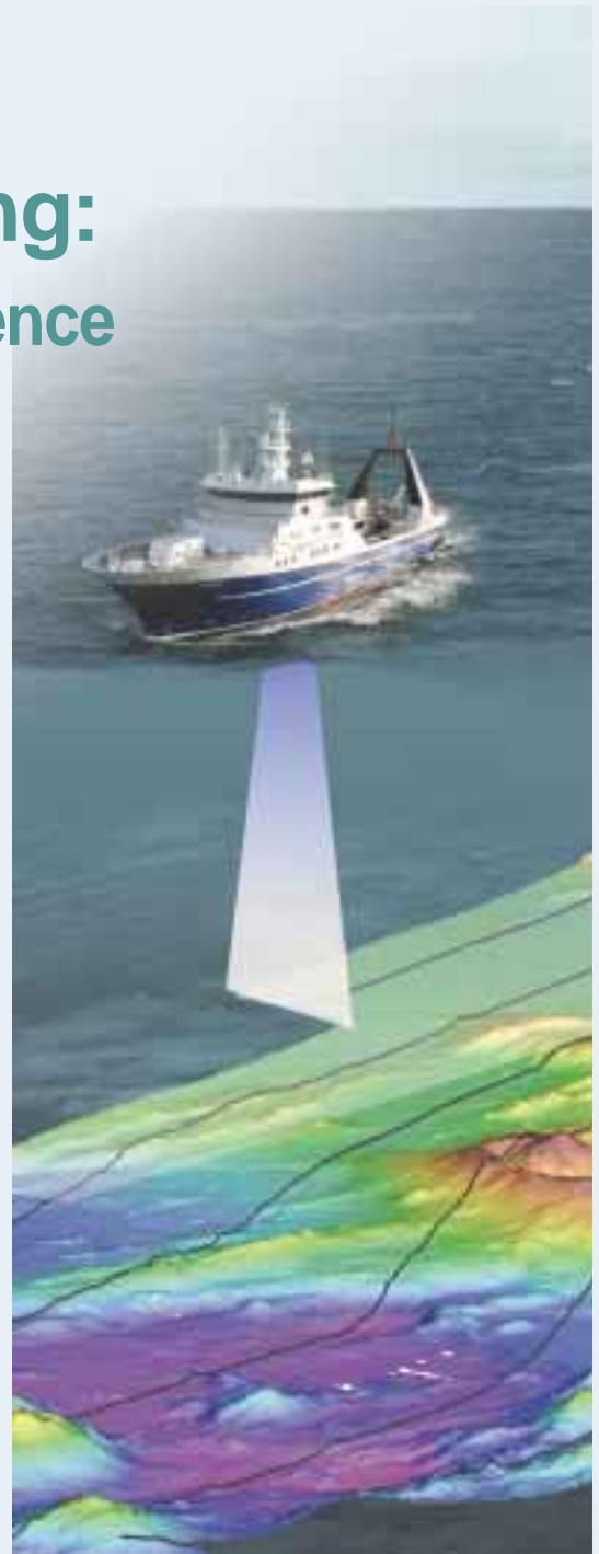
EM300 Multibeam surveys by R.V. Tangaroa . The black lines indicate the traverses of the vessel, required to build to the image.
