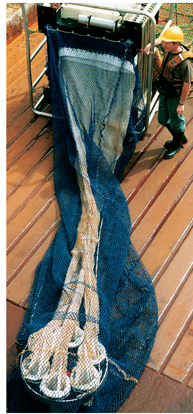
Russ Bradford with the multiple codend device secured to the end of the 60-m long fine-meshed net. (Photos: John Booth)
