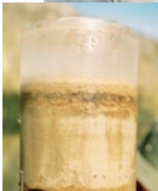
Sectioning a sediment core taken from Lake Gunn, Fiordland. (Photo: Ian Hawes) inset: close-up of the sediment core. Note layering of the sediments.
