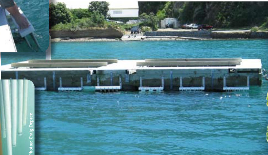
To field-test the formulations, Mike Tait lowers treated and untreated (control) fibreglass rods (shown below, left) over the side of the raft. The rods at right show the effects of fouling after 150 days in the water. In this trial, only the treated rod on the far right was free of fouling.
