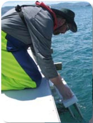
To field-test the formulations, Mike Tait lowers treated and untreated (control) fibreglass rods (shown below, left) over the side of the raft. The rods at right show the effects of fouling after 150 days in the water. In this trial, only the treated rod on the far right was free of fouling.
