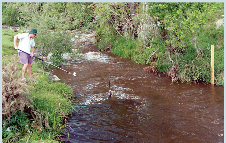
below: The front of one of the artificial flood events on the Topehaehae Stream. Richard Muirhead is about to take a sample for bacterial analysis. (Photo: Rob Davies-Colley)
