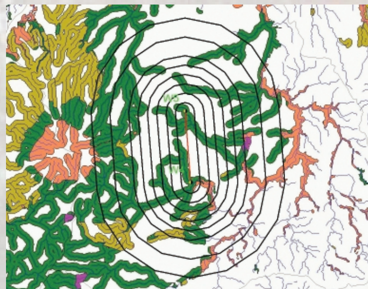
Example of riparian strips mapped around two of the study sites. The superimposed polygons were used in determining a "representative scale" for measuring the data set.
