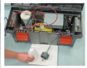
The CSM is portable, easy-to-use and gives quick readings. It fires a jet of water at the sediment surface in short pulses. The force of the jet is progressively increased until the erosion threshold is crossed. The CSM is used to survey sediments throughout estuaries and at different times of the year to assess spatial and temporal variability in sediment erodibility.
