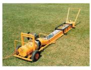
The NIWA submersible in-situ flume gives more detailed results than the CSM. It is shaped like an inverted "U", and is equipped with optical backscatter sensors, photodetectors, a water sampler and a current meter. As in the Waikato recirculating flume, water is accelerated through the flume by a propeller. Since the NIWA flume has no bottom, measurements can be
