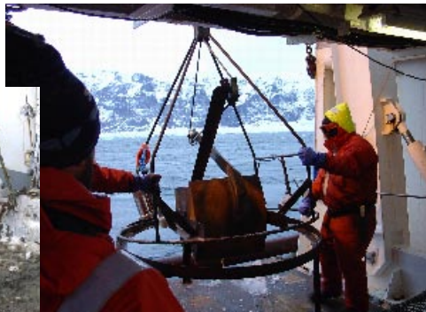
and a van Veen grab is deployed over the side. (Photos: Inigo Everson, BAS)
