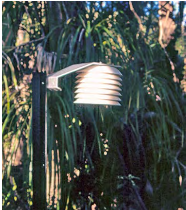
Figure 5.18: Microclimate data loggers mounted in a slotted conical cover to provide shade and relatively unimpeded air flow.
