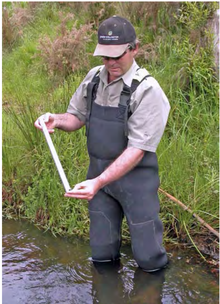
Figure 5.10: Using the “Wolman stick”. Photo: Richard Storey
