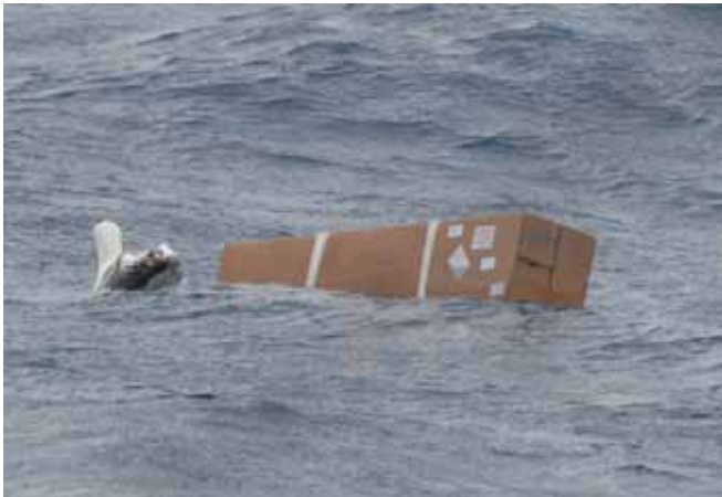
Fig. 5. Argo float after deployment over the stern of the vessel, in its fully biodegradable packaging material. This ensures maximum protection for the float during deployment.
