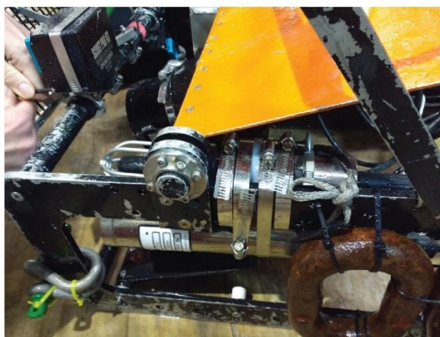
Figure 6-18 Hydrophone on camera frame exp. 20180718 (left) and hydrophone and RBR on camera frame exp. 20180718(right)
