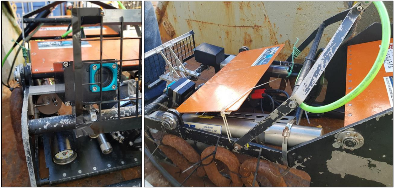
Figure 6-33 The IMAS Tow Camera with RBR sensor (left) and SBE 37 (right).
