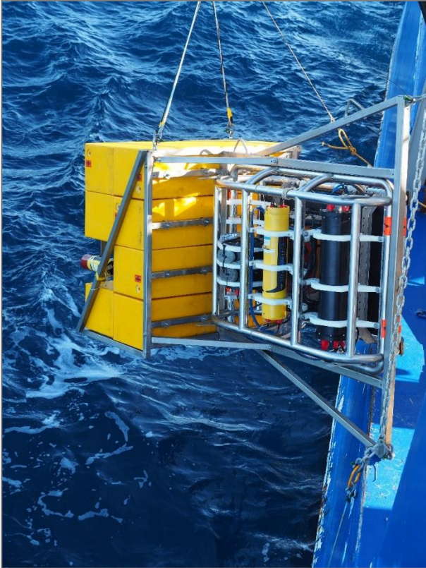
Figure 5-4 - AOS being lowered into the water.
