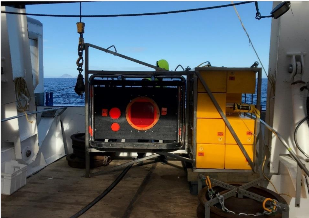
Figure 5-2 AOS fitted to the frame on deck ready for deployment. The two sets of bottom weights are also visible.
