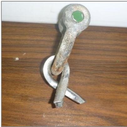
Figure 5-5 - Shackle with a badly deformed thimble.
