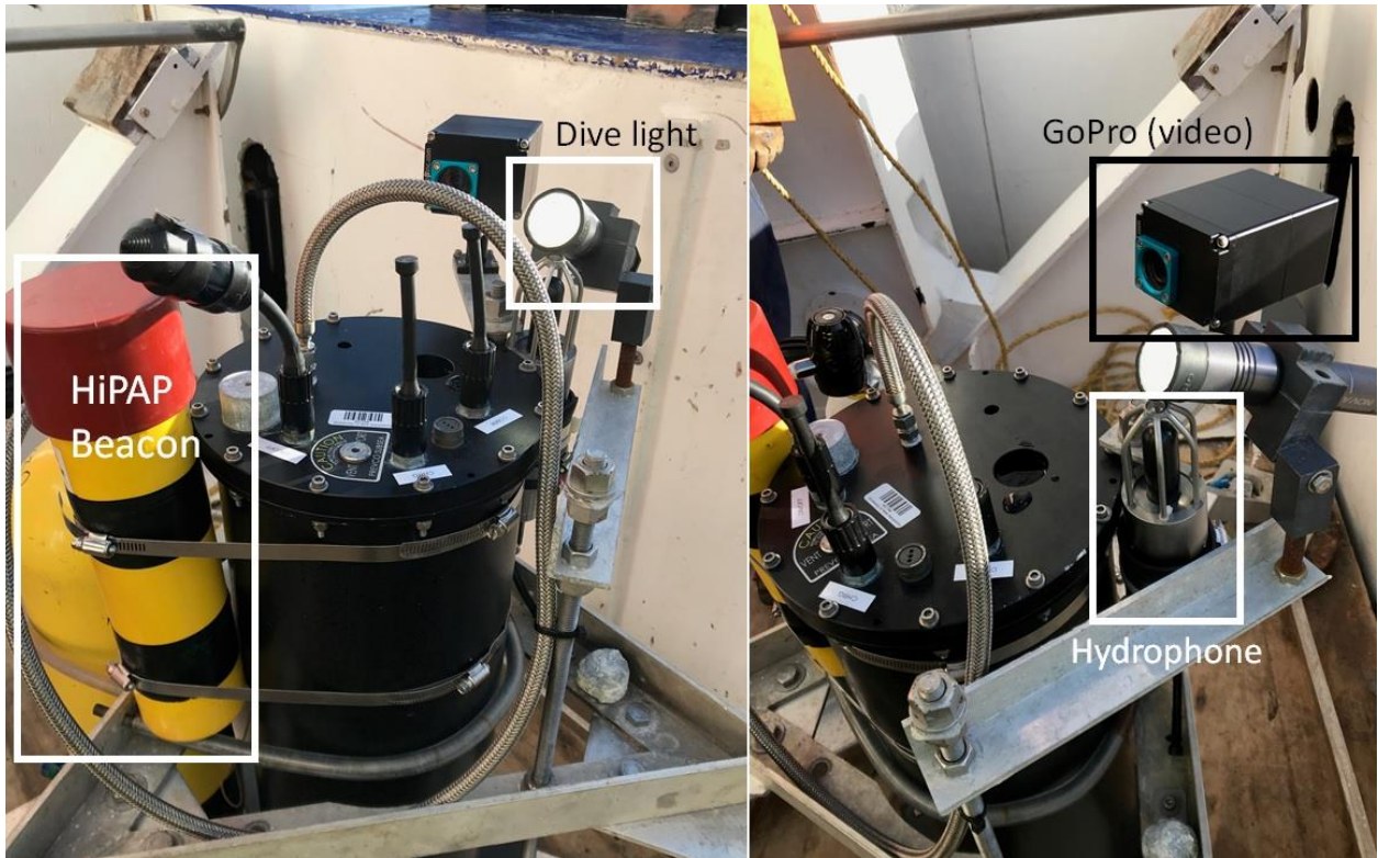
Figure 5-10. Auxiliary equipment employed during bubble maker operations: positioning beacon, video camera/dive light, and hydrophone.
