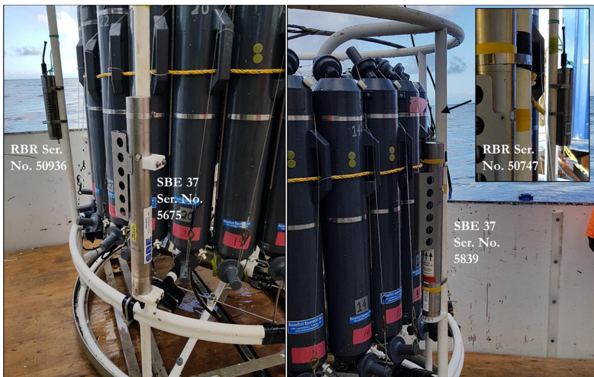
Figure 6-32 Two SBE 37 CTD probes and two RBR TD probes mounted on the CTD rosette.
