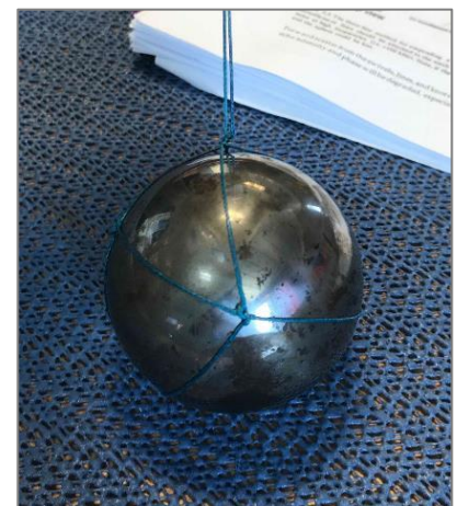
Figure 4-2 - making a sphere cradle for the calibration sphere
