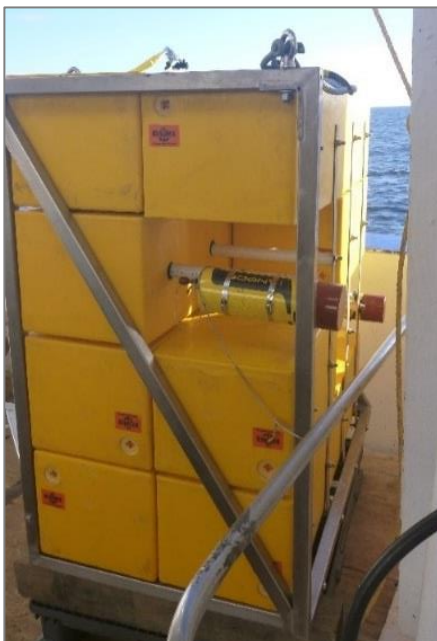
Figure 5-3 - The two HiPAP beacons secured to the frame.
