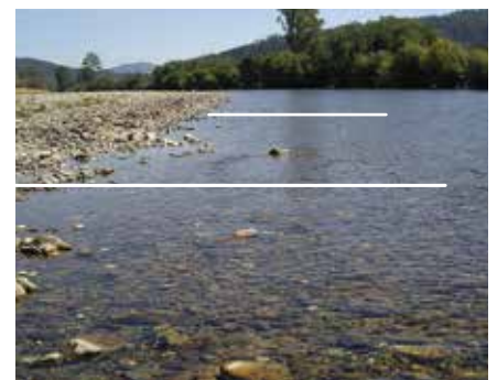
Larger (>15 m wide) and/or partially unwadeable streams (deeper than about 0.6 m): 2–4 transects extending partway across river. Space observation points evenly across transect.
