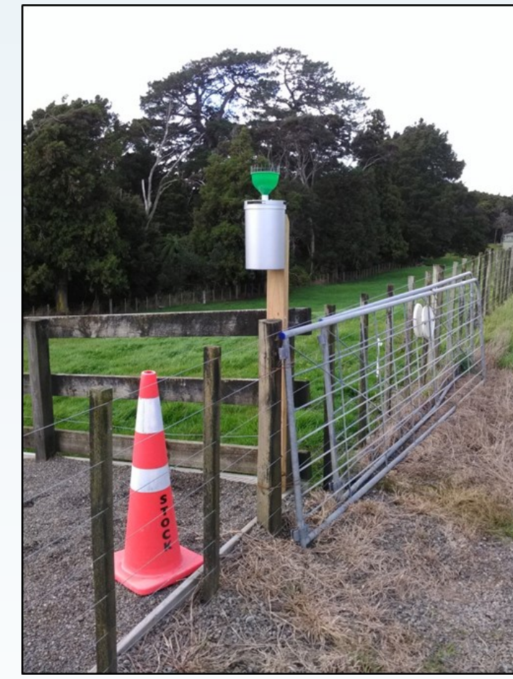
Figure 6 Stable isotope rain collector installed at Tututotara, Porewa.
