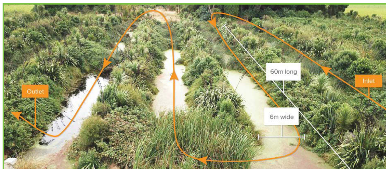
Photo shows serpentine flow-path though one section of the wetland. Shallower water depths would likely provide improved plant establishment and cover. Graphic courtesy of John-Paul Pratt (Groundtruth Ltd) and Neville Fisher (Kaiwaiwai Dairies).
