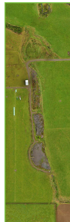
Newly constructed and planted wetland (left) showing direction of flow through initial deep sedimentation pond and subsequent two shallow elongated cells. Plant cover after one year shown on the right.
