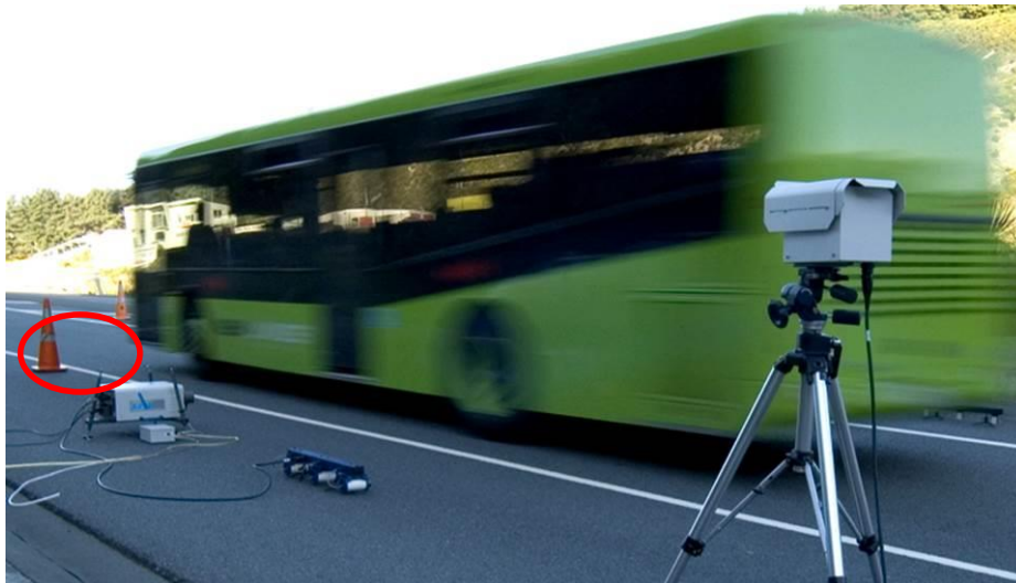
Figure 3-14: Speed bar (red circle) used for NZ remote sensing measurements.
