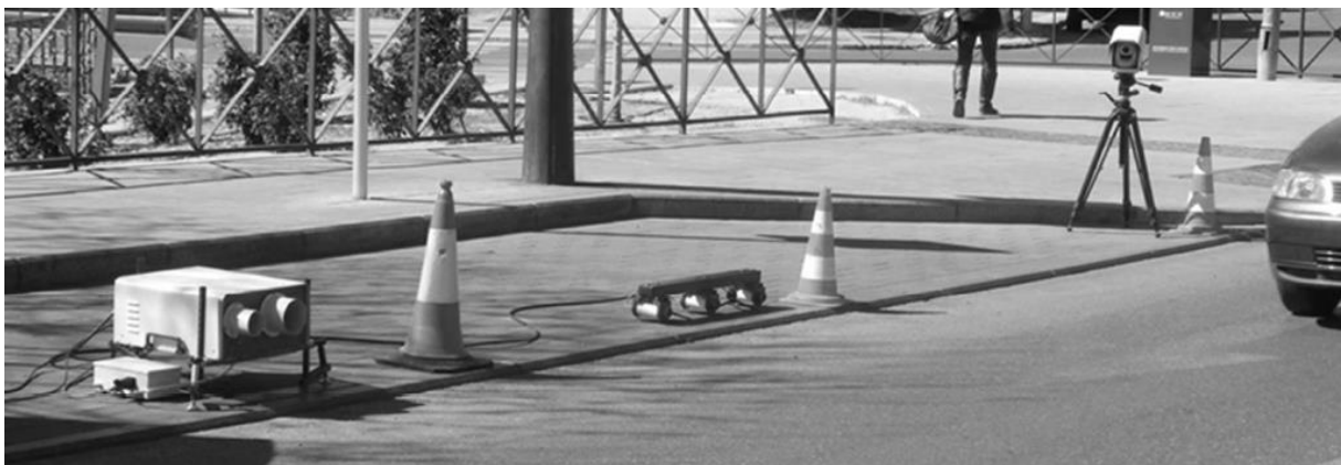
Figure 3-2: Photo of remote sensing measurement setup including speed/acceleration bar and a digital camera. (Source: Gala and De la Fuente, 2012)
