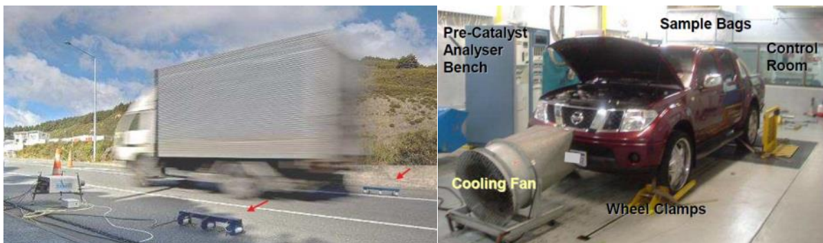
Figure 3-10: On-Road versus Laboratory measurements.
