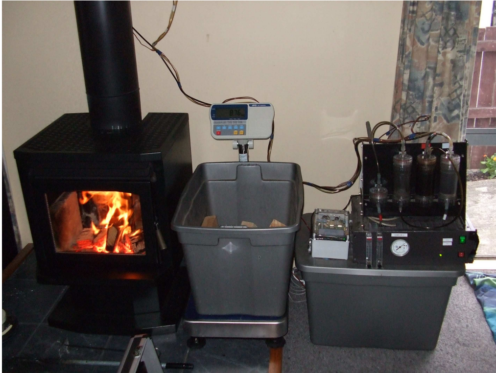
Figure 4-2: PM 10 sampler (at right) for in situ woodburner emissions testing
