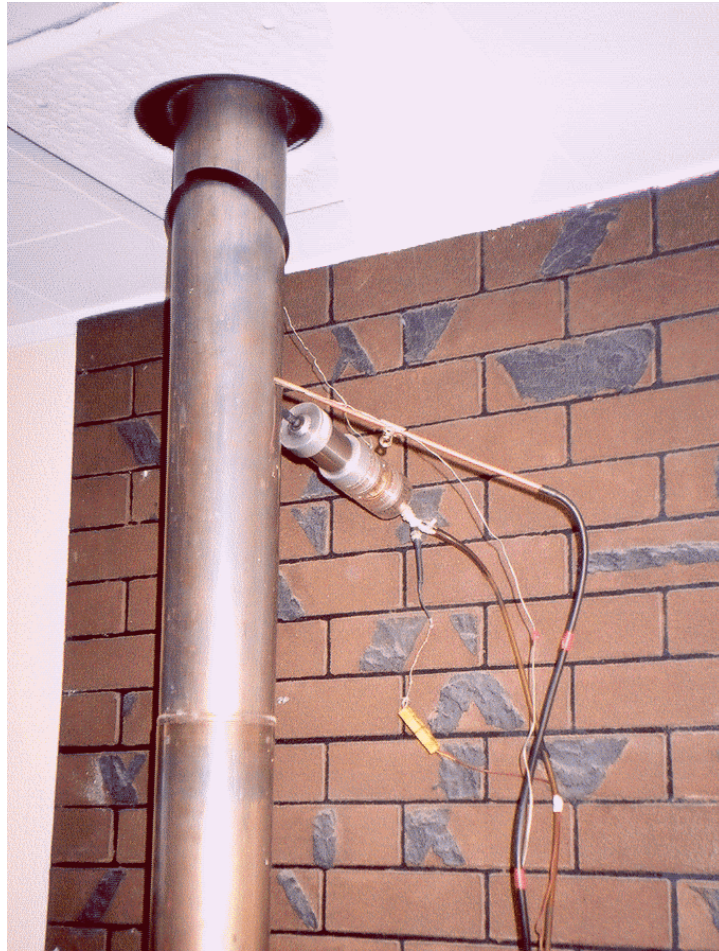
Figure 4-1: Flue intakes showing plain sample tube for gas analysis and manifold head for dilution sampling of PM 10 .
