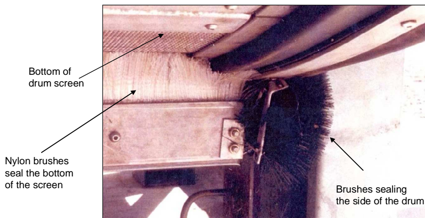
Figure 20: Use of brushes to seal the edges and sides of a revolving drum screens (from U.S. Department of the Interior 2006).
