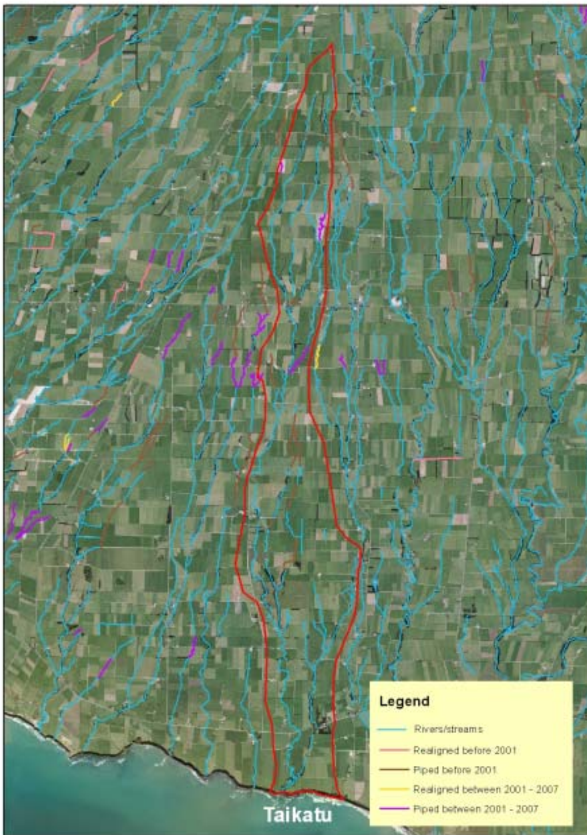
Figure 9 Mapped extent of stream modification in the Taikatu Stream catchment
