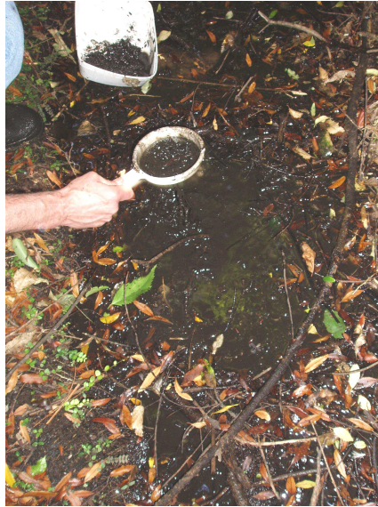
Figure 24. Step 1 in processing a sample: dump the contents of your sieve into a white ice cream box. Here, in dense bush in Dunedin, the samples were taken closer to abundant clean water and brighter light for subsequent steps.
