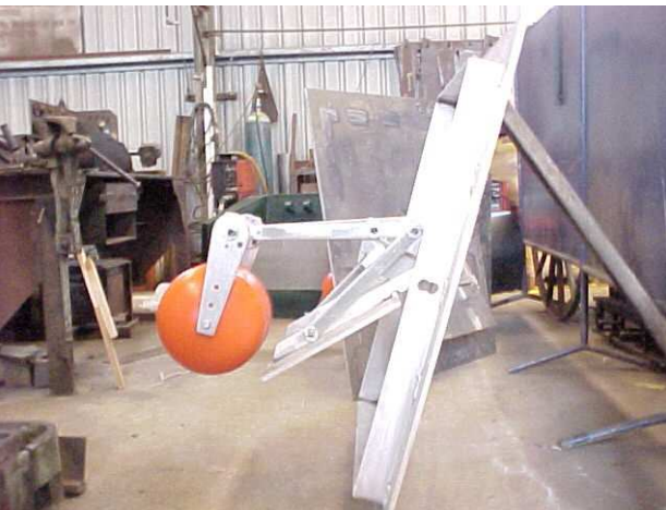
Plate 9 : Upstream tidally operated floodgate
