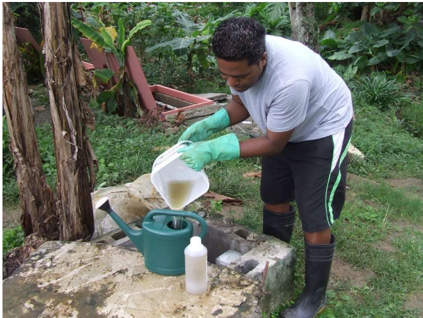
Figure 4-4: Septic tank effluent being collected from the Flout chamber. The effluent was then manually sprinkled over a section of the LAS sand filters to simulate a dosing cycle. The filtrate emerging at the base of the sand bed was later collected via the Fullstop™ samplers.
