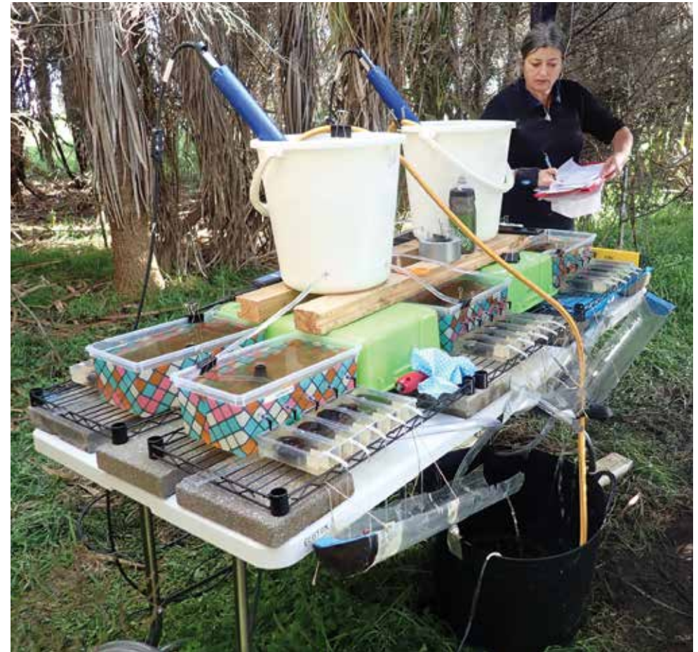
Recirculating flow-through experimental system for testing kākahi clearance of E. coli bacteria from lake water.
