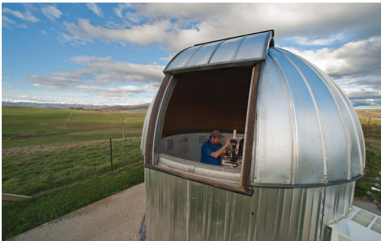
NIWA Science Technician Hamish Chisholm uses a Dobson spectrometer to measure ozone above Lauder. The spectrometer measures the total ozone column (effectively the thickness of the ozone layer as a column through the atmosphere) using either a direct sun measurement or a zenith measurement. The thickness of the ozone layer is measured in Dobson Units (DU). Values at Lauder typically range between 230 and 400 DU, with the highest values recorded in spring. (Dave Hansford)
