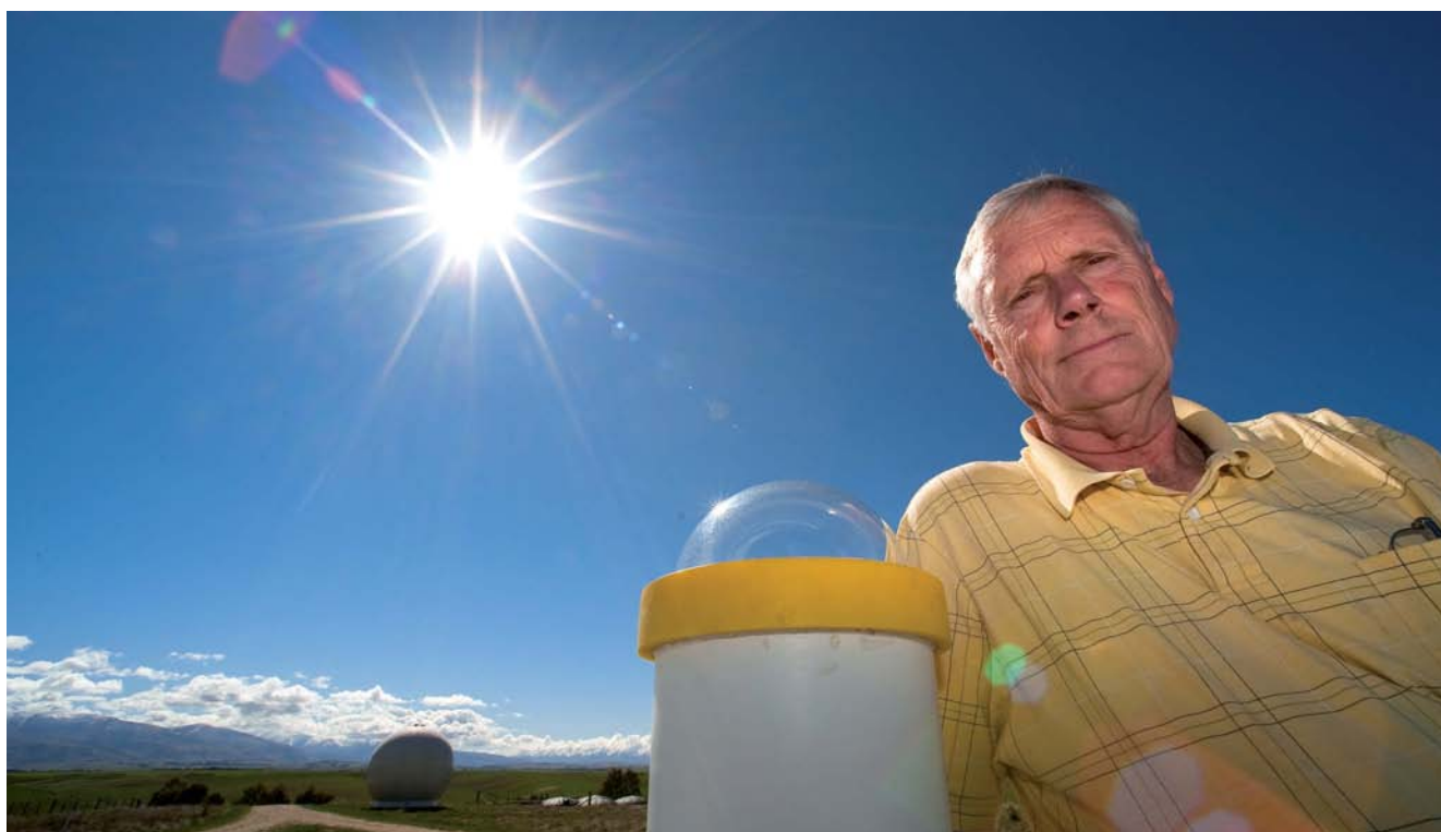
NIWA Atmospheric Scientist Emeritus, Dr Richard McKenzie, with an all-sky camera at the Lauder Atmospheric Research Station in Central Otago. The device, owned by the University of Hannover in Germany, takes a high-resolution picture of the full sky every minute, building the long-term record of cloud cover essential to our understanding of UV radiation. [Dave Hansford]
