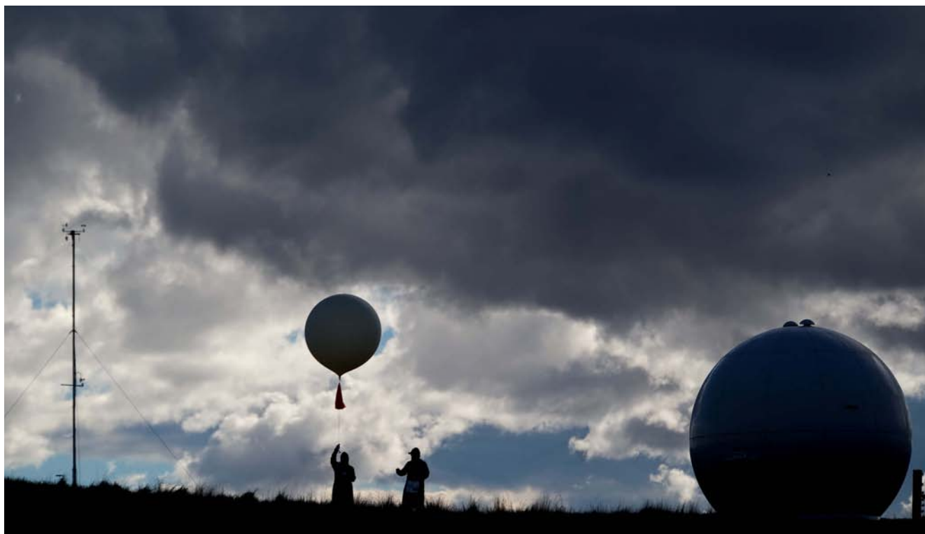
Technicians release a balloon at Lauder. Chemical sensors attached will measure the vertical ozone profile up to an altitude of around 35 kilometres before descending. (Dave Hansford)
