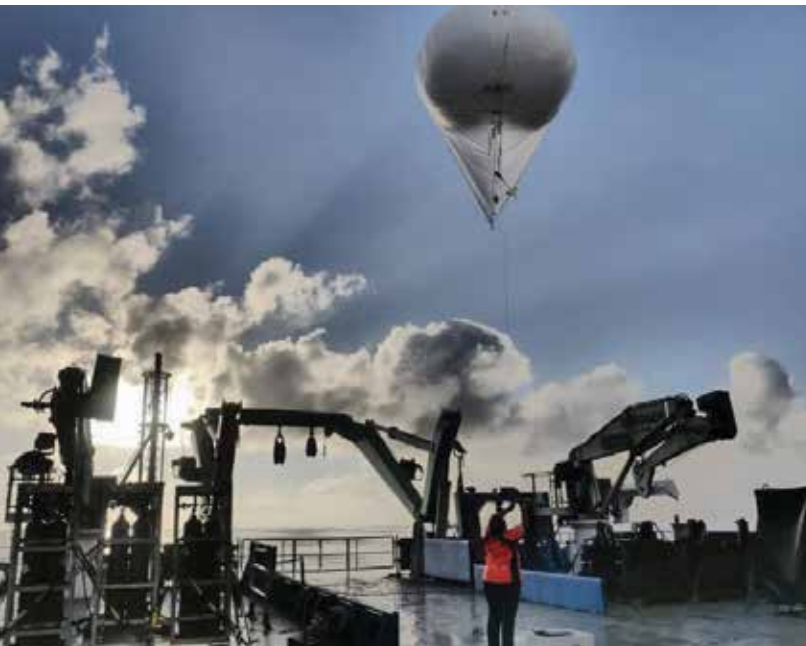
A helikite is deployed from CSIRO's research vessel the Investigator to measure temperature, humidity, wind speed, wind direction and atmospheric pressure. (Tony Bromley)
