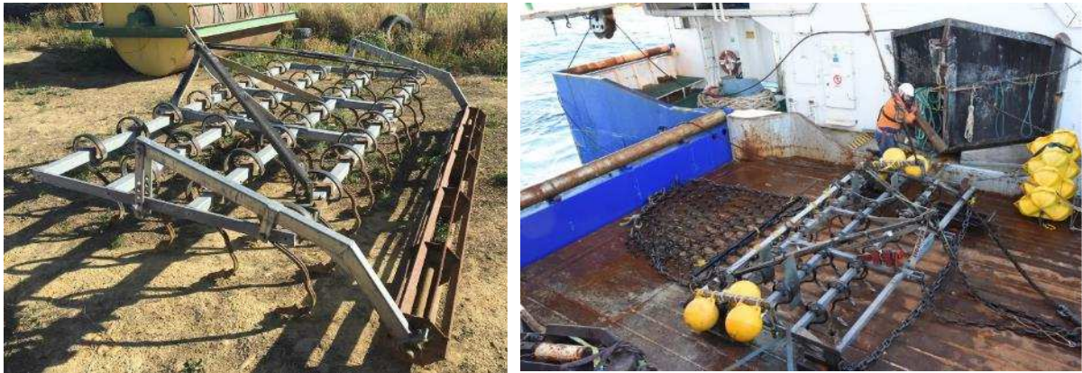
Figure 4-10: Images of SCIP, showing the roller configuration (left) and final harrow mat configuration (right).
