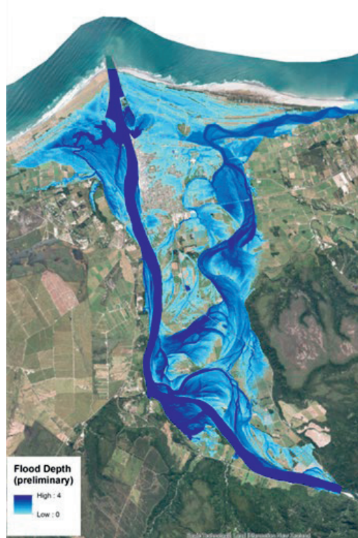
Model of flood inundation in Westport that accurately replicated the actual July flood event of the Buller River.
