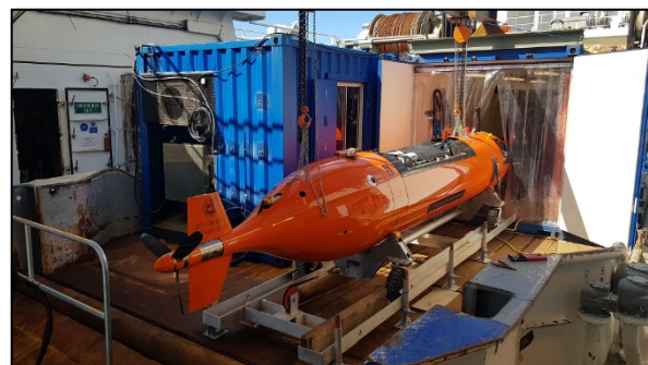
Installation of the 9.5-m-long launch and recovery system on the Tangaroa trawl ramp (left), and the AUV on deck with the workshop and control containers (right).
