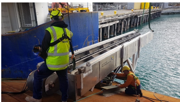
Installation of the 9.5-m-long launch and recovery system on the Tangaroa trawl ramp (left), and the AUV on deck with the workshop and control containers (right).
