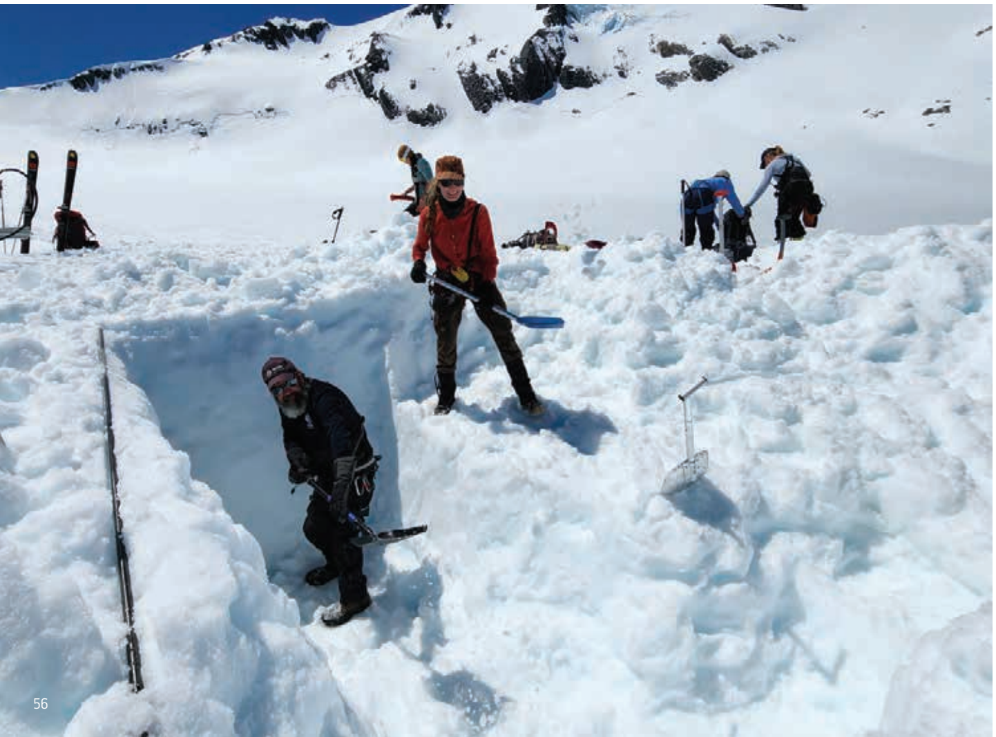
Principal Scientist – Climate and Environmental Applications Dr Andrew Lorrey and University of Otago colleagues dig a snowpit on Brewster Glacier for mass balance monitoring. [Gregor Macara]
