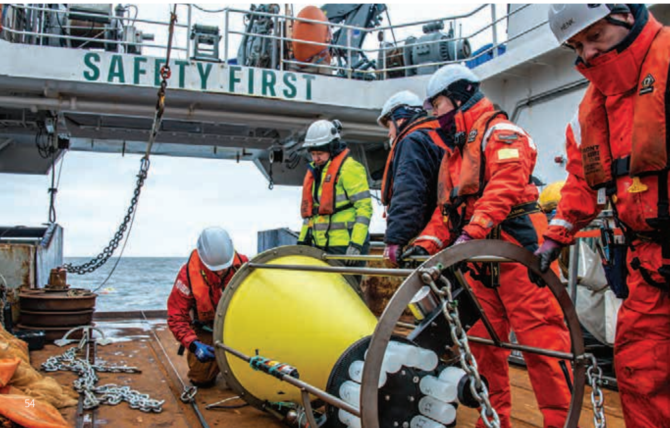
| Researchers work with crew onboard RV Tangaroa to prepare a sediment trap mooring for deployment to recover deepsea samples from the Southern Ocean seafloor. [Joshu Mountjoy]
