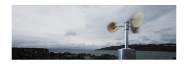
Wind speed is often measured in kilometres per hour (km/h) or metres per second (m/s) and scientists often use a tool called an anemometer to measure the speed.
