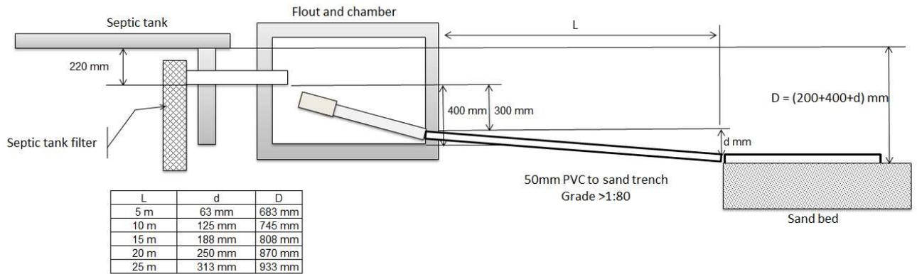
**11.5 DRAWINGS D5: DOSE LOADED RAISED SAND FILTER TRENCH**
