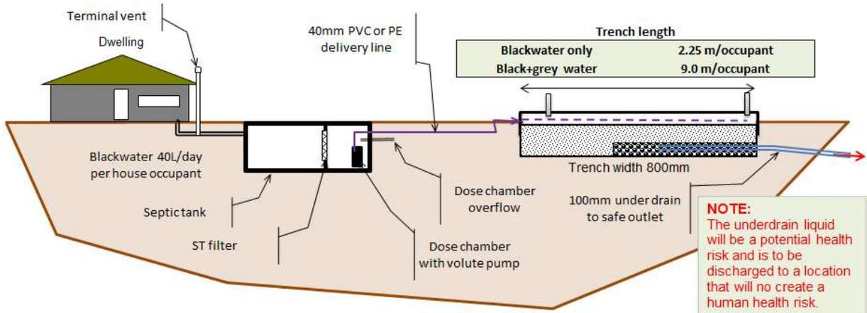
Drawing D6.2. Gravity (Flout) dose loading to a sand filter trench with under-drain.
