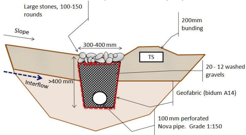
**Drawing D6.4. Cross-section of sand filter trench with under-drain**
