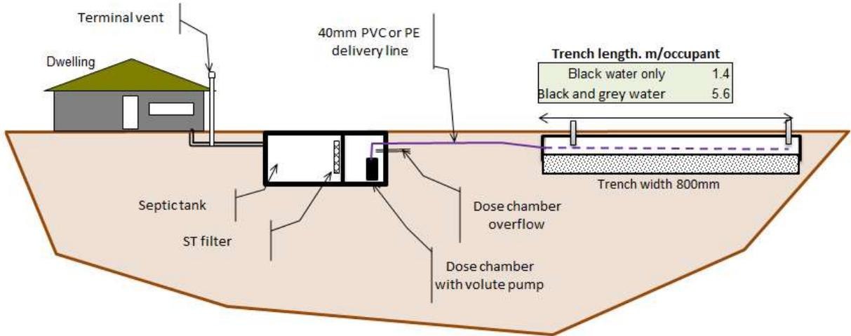
Drawing D4.3. Cross-section of sand trench on free-draining soils
