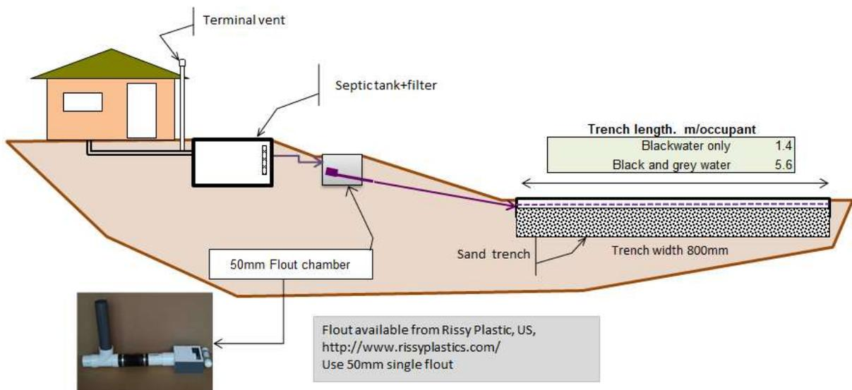
Drawing D4.2 Alternative pump dose loaded sand filter trench
