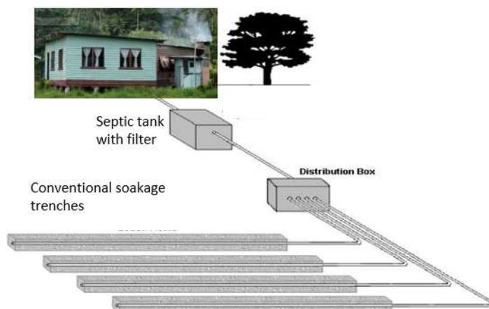
For both free-draining and moderately-draining soils, Table 1 provides the trench length required per occupant for a 600mm wide trench for both blackwater only and for combined black and greywater systems.
