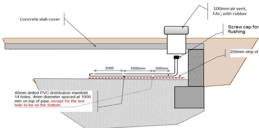
Refer to **Drawings D5.2 and D5.3** for plan details of the distribution pipe and flushing requirements.
