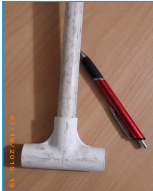
Photo 4. PVC tee fixed to the end of a length (at least 2.5 m) of 15mm PVC pipe to form a probing rod.
