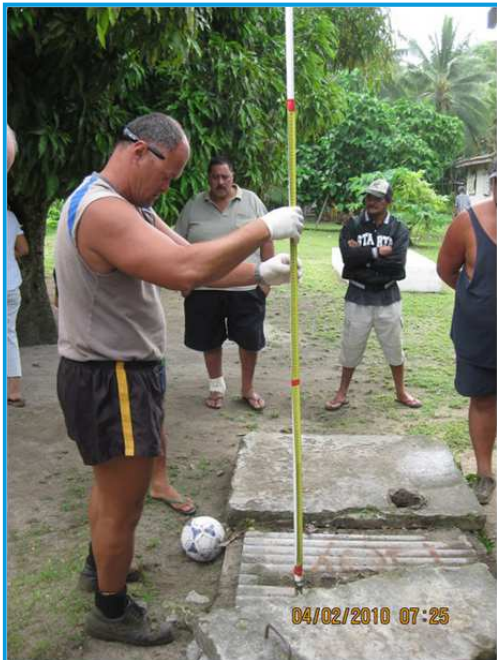
Photo 3. Probing septic tank first chamber for scum and sludge depth.
